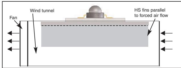
**Figure 3.E. Finned Horz. in Wind Tunnel**
