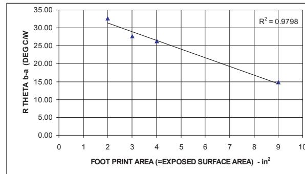
Flat Heat Sink, 0.09" (2.3 mm) Horizontal on insulating foam
