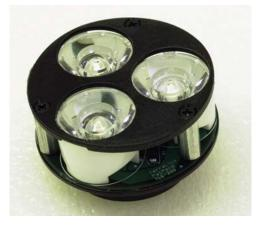
TerraLUX TLE-300, the World's Brightest Flashlight Upgrade, using LUXEON K2 with TFFC.
