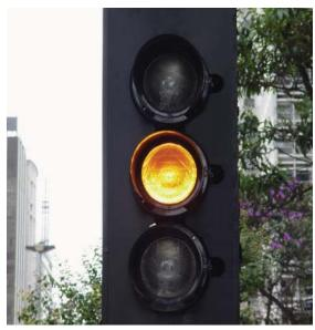
Meng Engenharia adapted the prototype to traffic light applications in a version containing seven LUXEON I LEDs per bulb, a built-in power supply, and the standard E-27 screw-in base used in South America. The distribution of the LEDs across the bulb was designed to replicate the basic radiation pattern of an incandescent bulb filament. The LEDs were positioned to work with the existing reflector inside the traffic light head to avoid the expense of reflector replacement.
