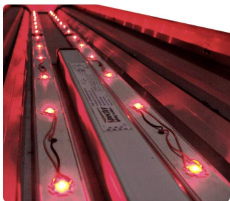
**One of 3,000 light boxes built for the project, using 875 different types of assemblies consisting of 2 to 32 LEDs**
